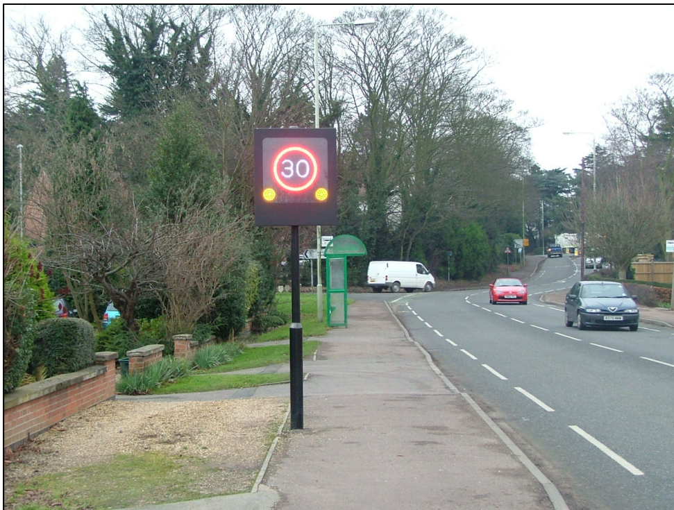
A Vehicle Activated Sign displaying a 30 mph warning when triggered by vehicles travelling at excessive speed.
